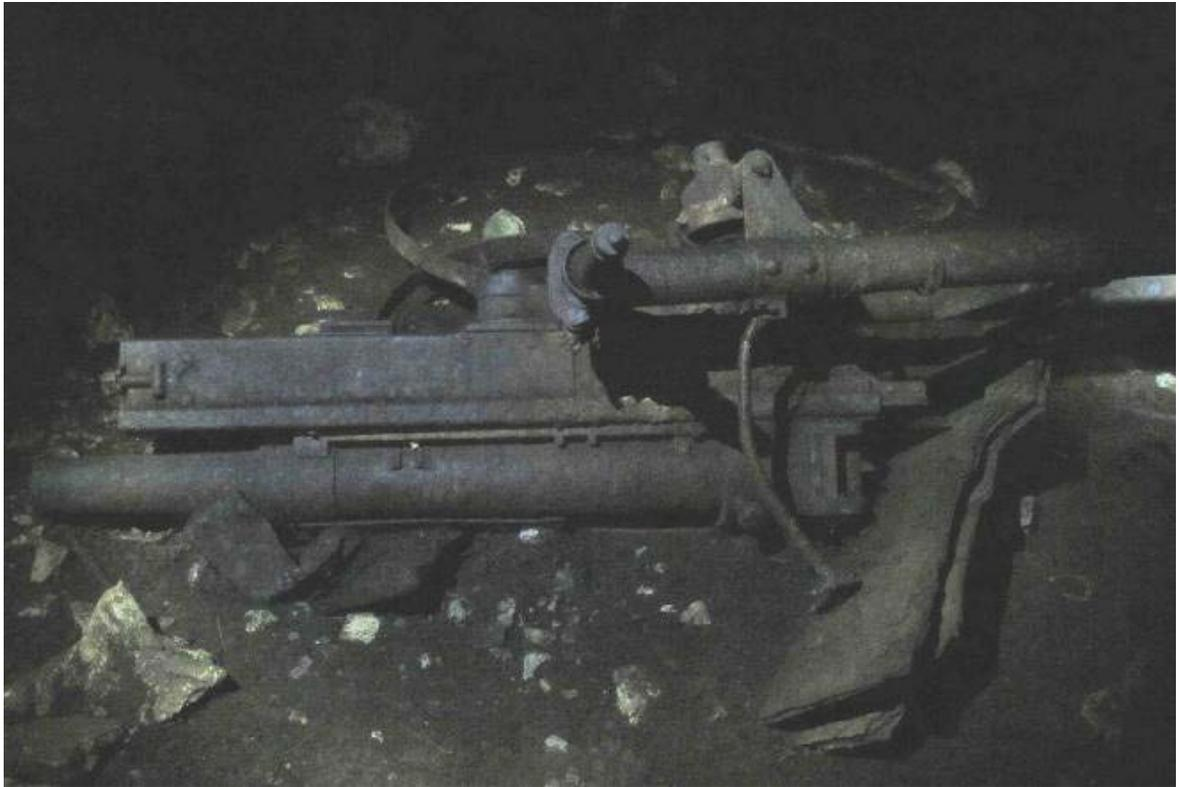
**Figure 6.36** Japanese 75mm gun which protected the eastern mouth to the Japanese Navy Command cave, now upside down on the cave floor after being hit by American fire.
