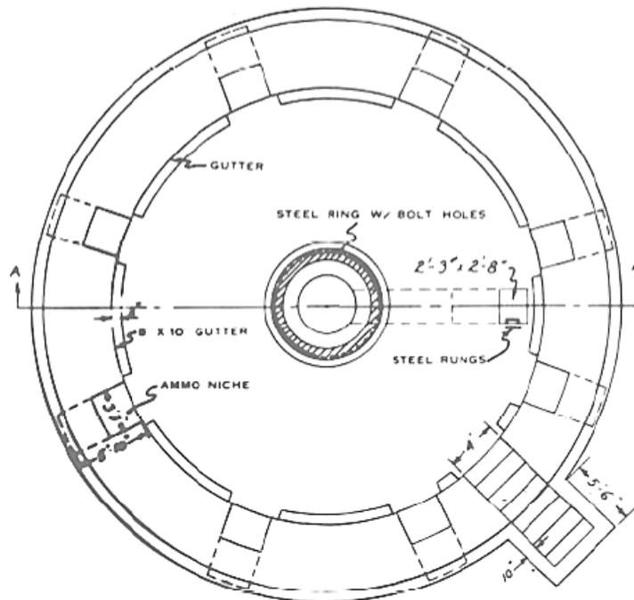
**Figure 4.31** Plan diagram of Japanese 127 mm gun emplacement (First Marines 1944)
