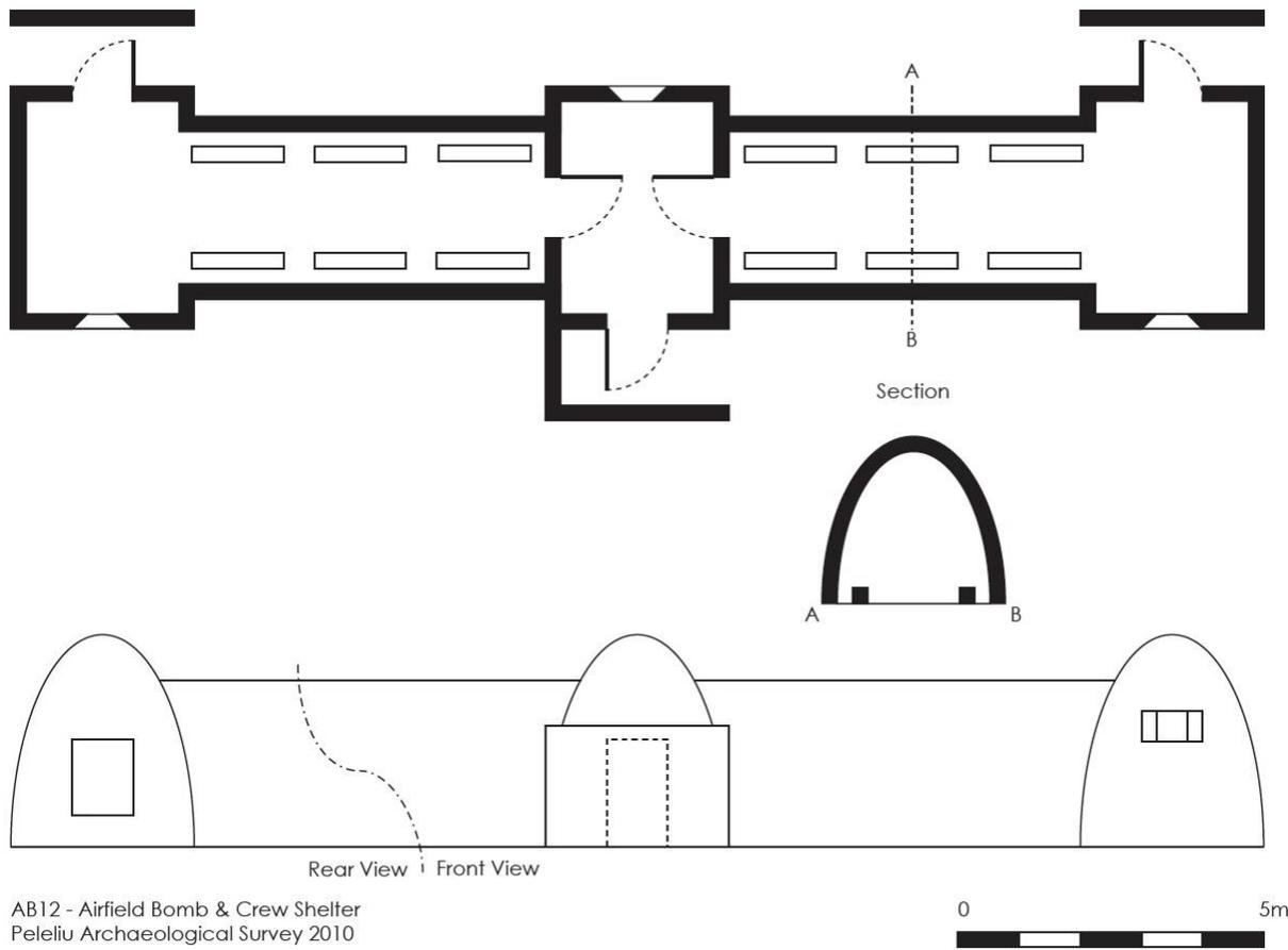
**Figure 5.26** Plan view of the long concrete bomb shelters exemplified at AB12. (drawing by Gavin Lindsay)
