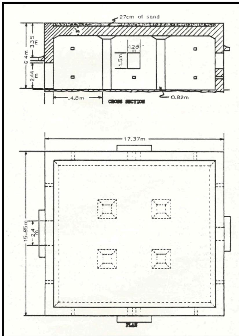
**Figure 3.27** Plan of a concrete Japanese fuel bunker similar to AB168 (After Denfeld and Russell 1984). The AB168 building may have never held fuel and Marines found miscellaneous machinery inside when the building was secured.
