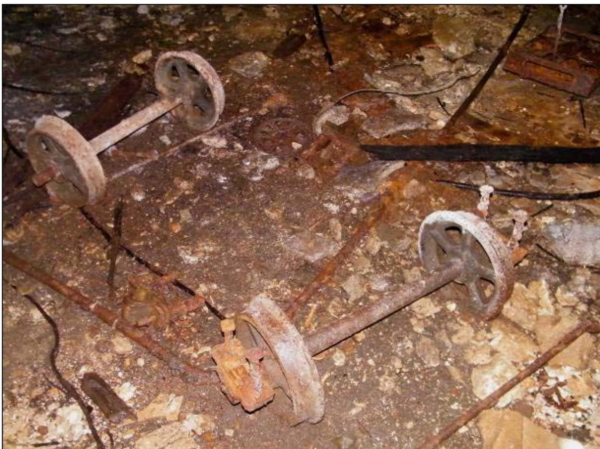
**Figure 6.27** Remains of one of the narrow gauge rail cars salvaged from the phosphate mines on Peleliu and reused by the Japanese military. Only the wooden elements are missing.
