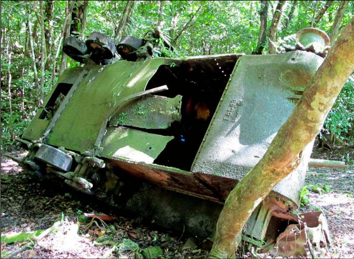
**Figure 6.66** The bottom of the Sherman tank at AB270, showing damage from the buried Japanese bomb that it ran over.
