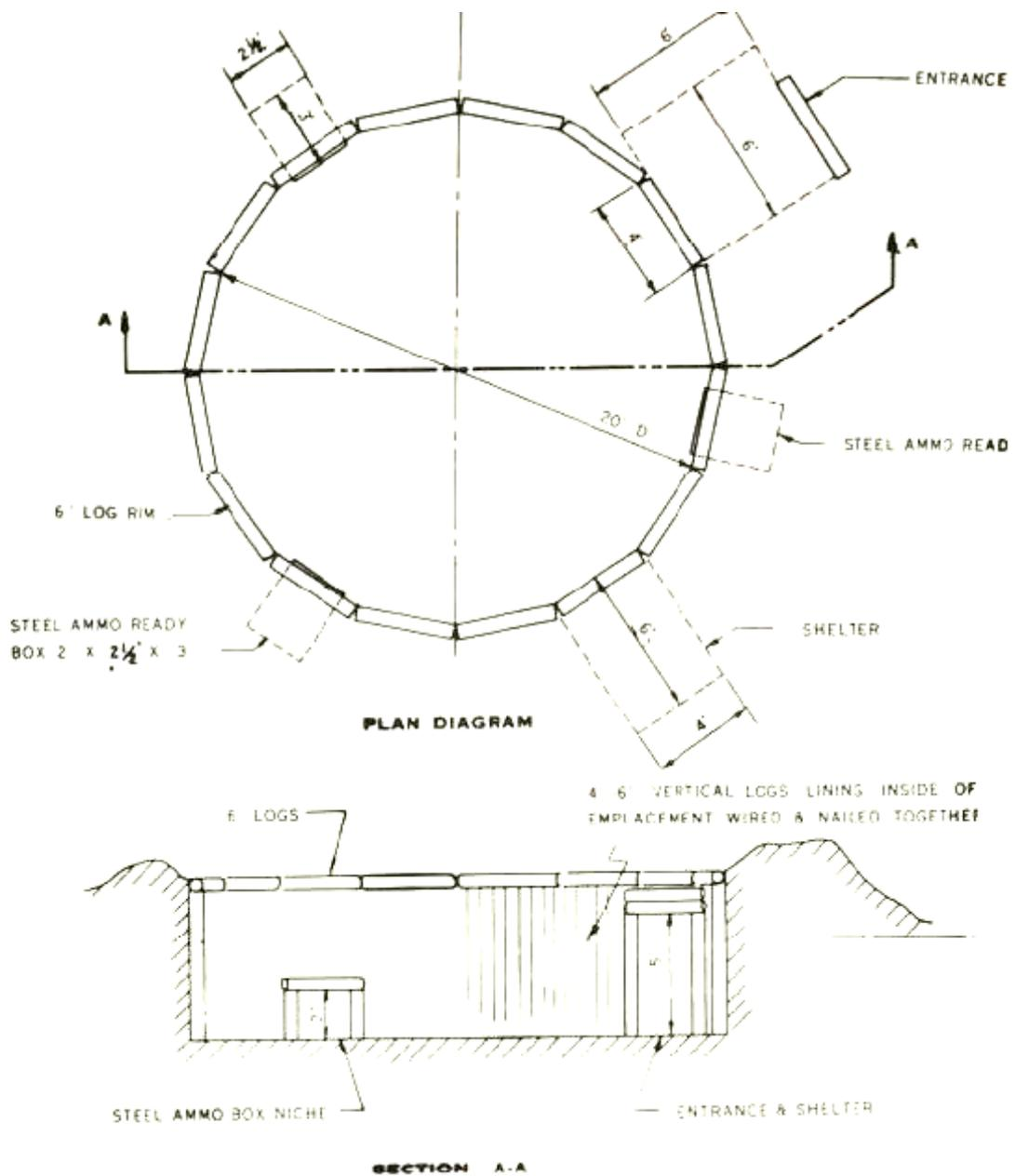
**Figure 4.27** Plan diagram for the Japanese 120 mm gun emplacement at AB187 as it was documented in 1944 (First Marines 1944).
