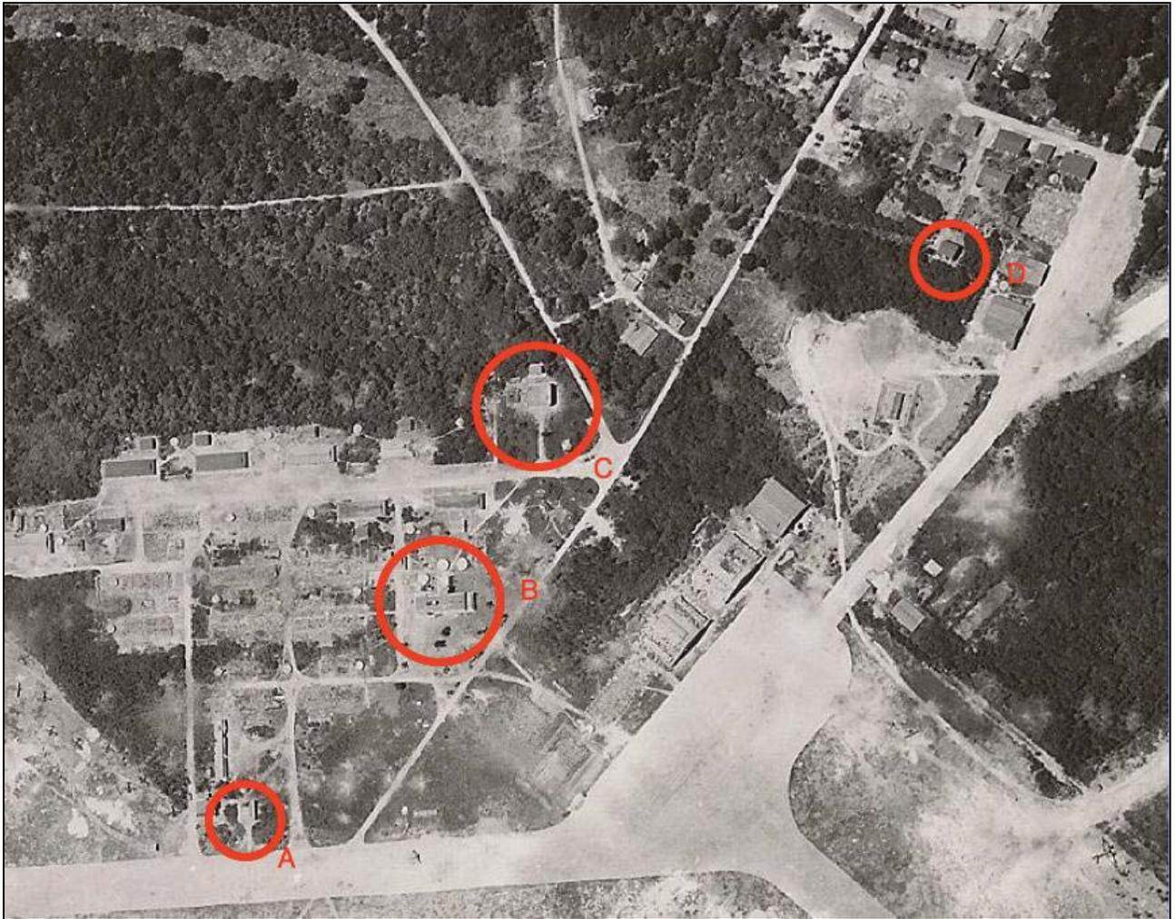
**Figure 5.49** Detail of Peleliu airfield in March 1944, with the largest surviving Japanese structures circled: A; Air operations building (AB262), B; Air Headquarters building (AB38), C; Main power plant (AB36), D; Power plant 2 (AB32). (NARA: RG127)
