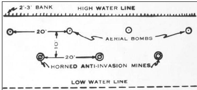
**Figure 3.8** Diagram of mine layouts found by Marines on White and Orange Beaches (after First Marines 1944:)
